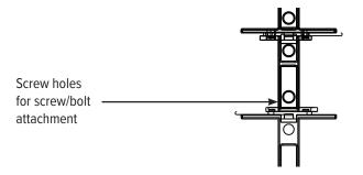
**For Wood:** Use wood screws to secure bird spike strips to wood surfaces. Using pre-drilled holes along the base, screw into the end of each bird spike strip tightly and place one wood screw at least every six inches along the base.
