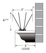
• For wide areas, multiple rows of bird spike strips may need to be installed. Install bird spike strips with 1" overlap.
