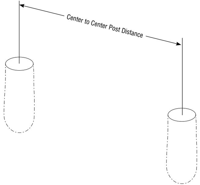
**3** If frost line exceeds 30" dig hole to the appropriate depth and then add 6" of gravel for post drainage. Add concrete according to manufacturers instructions until a depth of 30" remains. Set post in hole ensuring it is plumb and level. Fill hole with concrete according to manufacturers instructions. Go to step 5.
