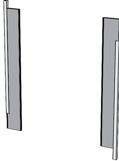
**7** Insert pickets/boards from left to right into lower rail(s) ensuring U-Channels are on both ends.
