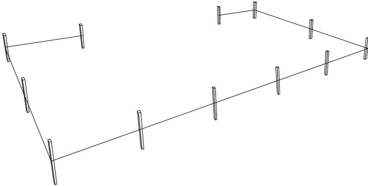
**2** Dig post holes 12" in diameter 36" deep. Use the Center to Center measurements of the fence model being installed for the Center to Center Post Distance. If a fence panel is being used that is less than the width of a full panel, or if posts are being used other than 5" in width, measure the width of the panel and add the width of one post, that will be the Center-to-Center post distance of the holes.
