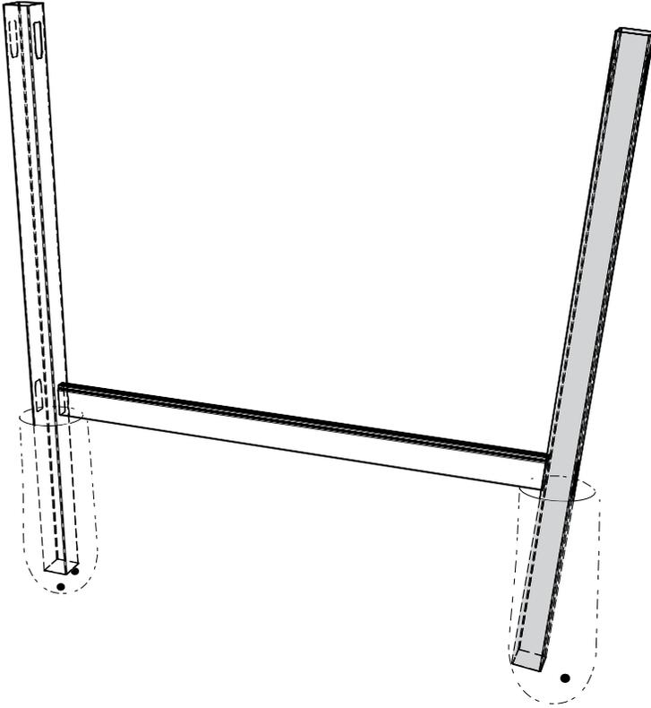
**6** Next, attach U-Channels to boards (If applicable). If assembling Red Cedar panels, you must screw U-Channels to post first and then add boards.
