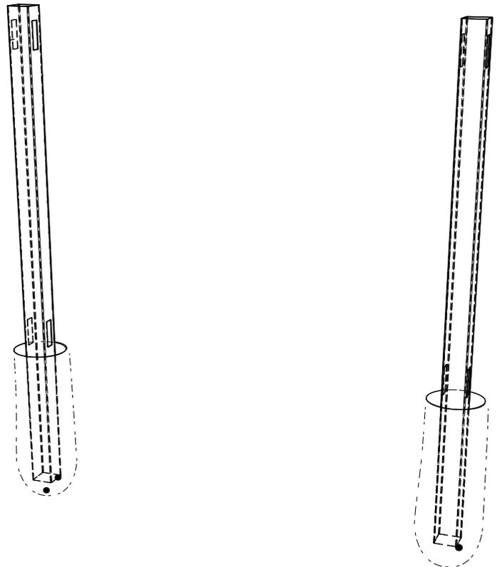
**5** For Build-It-Yourself panel, insert aluminum into bottom rail, then insert bottom rail into bottom post route hole of first post only.
