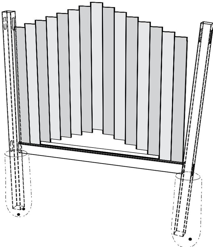
**8** Insert the top rail into the left side of the post route then guide over top of pickets/boards.
