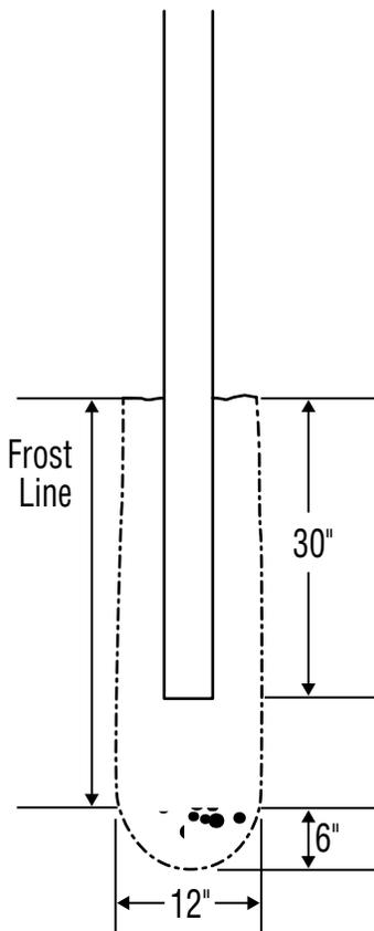
**4** If frost line does not exceed 30", insert 6" of gravel into bottom of both holes then set post in ground ensuring it is level. Ensure first post is plumb and level and then add concrete according to manufacturers instructions.
