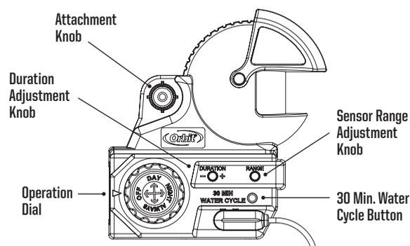
The sensor detects the combination of both heat and movement to activate the valve.
