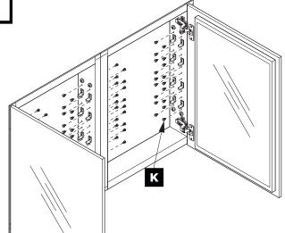
Fill the remaining holes with a plugs (K).
