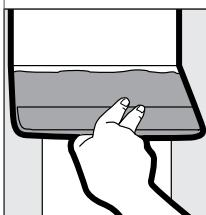
Allow joints' second coat to dry overnight. If necessary, remove imperfections with knife or sandpaper. Apply a thin finishing coat of all purpose or topping compound with a 10 in. or 12 in. knife. Press knife firmly so joint compound fills depressions but does not significantly add to thickness. Feather edges at least 2 in. beyond second coat. Allow third coat to dry overnight.
