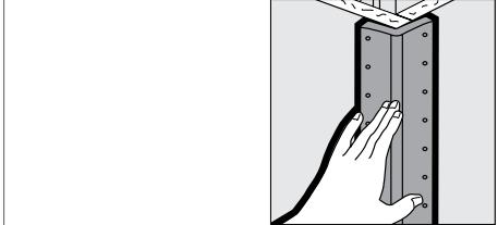
Drive all mechanical fasteners below nose of corner bead. Be careful not to dent the metal.\*
