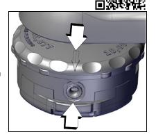
Insert one end of trimmer line into an eyelet, and push line equal distance through trimmer head.
