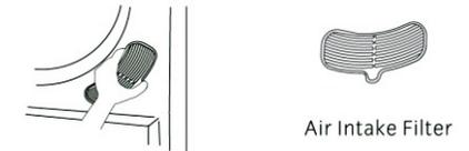
Slightly push upwards with your thumb until the latch hook disconnects, then remove.
