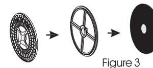
Note: The filter fixed in the bottom of the drum should also be cleaned with a soft brush.
