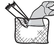
Ensure that foreign objects do not find their way into the dryer. All pockets should be emptied, buttons, buckles and zips fastened. This will also help reduce impact noise when the items hit against the turning drum.
