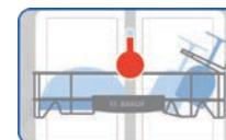
Final hot water wash increases the tub temp.
