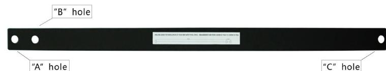
4. Continue around the entire pool, drill all holes using the drilling template for guidance. Place the "B" hole marked on the drilling template over the last hole drilled. (see figure 2), then drill through the "C" hole. Repeat this step for every 3.7 M (or at the end of each fence unit), you must also drill through the "A" hole to accommodate the pole from the new fence unit.
