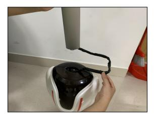
•Connect the car body wire terminal with the car battery wire terminal.
