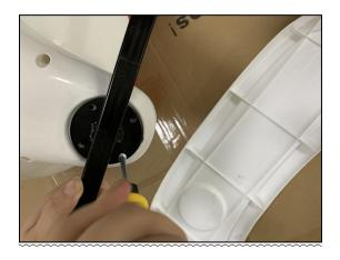
•When using the mobile seat independently, separate the car body from the seat, install the iron bar with a pair of wheels under the seat, and fix it with four Ø 4 \* 20 self tapping screws
