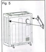
The appliance shall not be exhausted into a chimney, a wall, a ceiling, an attic, a crawl space, or a concealed space of a building.
