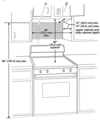
A. 2" x 4" (50.8 mm x 101.6 mm) wall stud B. Grounded 3 prong outlet
