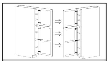
To reverse the door, unscrew the 3/4" round head phillips screws from each hinge and remove the door panel. Then, reverse the door panel and drill the 3/4" round head phillips screws to each hinge through the pre-drilled holes to tighten the hinges with cabinet face frame.
