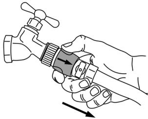
**10** Pull down blue quick connect sleeve to disconnect hose from hose bib adapter.
