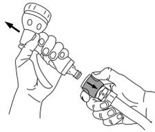
**2** Slide down blue sleeve to release quick connect from the nozzle.
