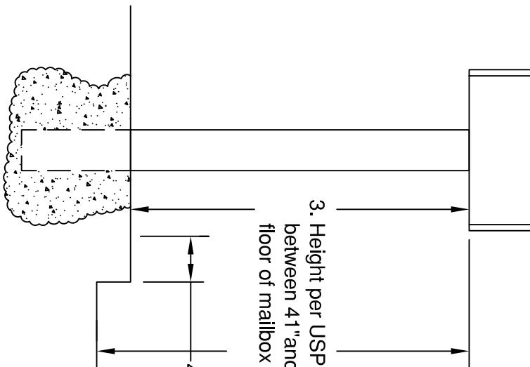
2. Customers are required to contact the local post office before installing the mailbox to ensure its correct placement and height at the street. Generally, mailboxes are installed at a height of 41-45 inches from the road surface to inside floor of the mailbox or point of mail entry (locked designs) and are set back 6-8 inches from front face of curb or road edge to the mailbox door.
