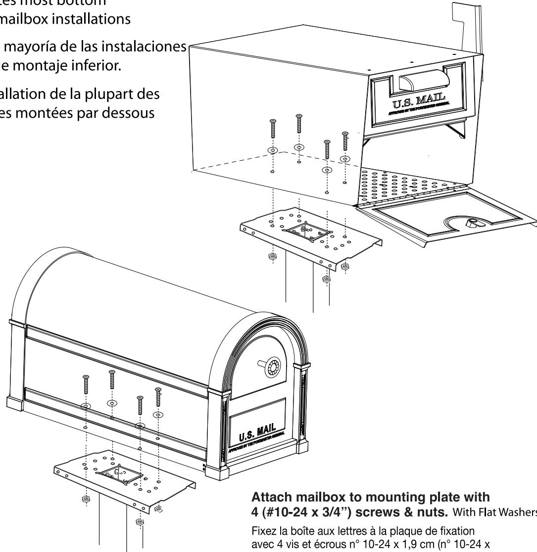
**Attach mailbox to mounting plate with 4 (#10-24 x 3/4") screws & nuts.** With Flat Washers
