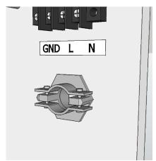
Once the wire has been run through the plate, you must connect the wire to the unit matching the colors of the inside wires. After the wiring has been completed return to the original installation procedures.
