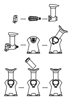
1. Put and lock the tray on chute top properly. Insert the grinder into the chute. Be sure the gasket is properly placed inside the dispenser. Then affix the dispenser to the chute by placing on the front and turning counterclockwise to lock.
