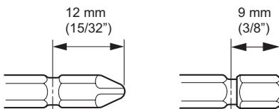
Use only the driver bit/socket bit shown in the figure. Do not use any other driver bit/socket bit.
