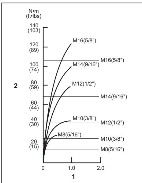
► 1. Fastening time (second) 2. Fastening torque
