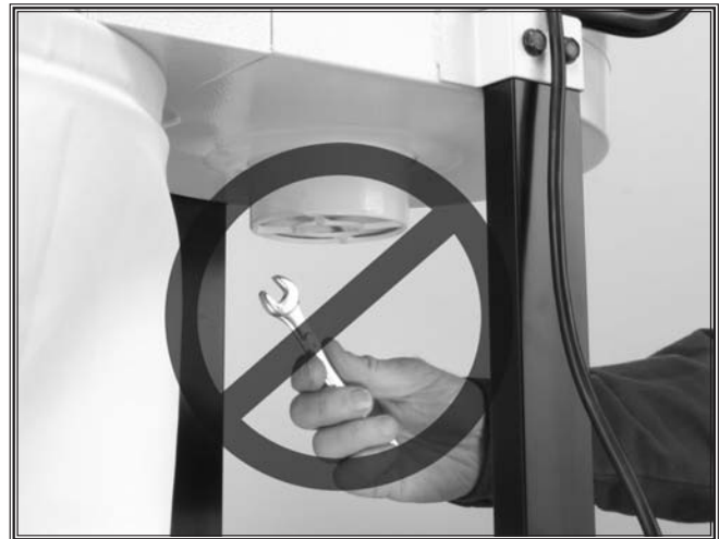
Figure 5. NEVER work around the intake port when the dust collector is operating.
