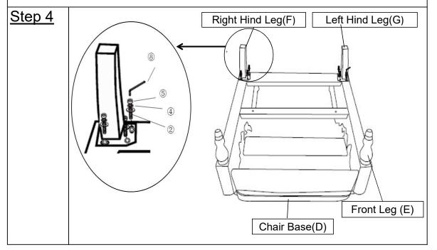
Attach the Right Hind Leg(F) and Left Hind Leg(G) to Chair Base(D) use Bolt(⑤), Washer Ring(④), Washer(②) with Allen Key(⑧) by turning the legs clockwise as shown.
