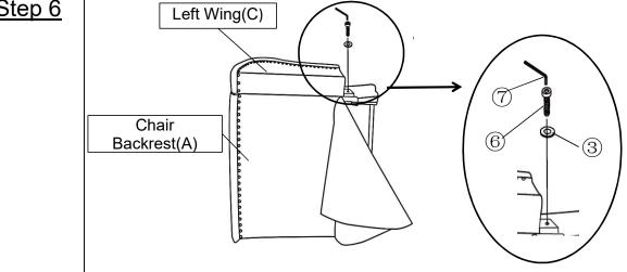
Attach Left Wing(C) to the Chair Backrest(A) using Bolts(6) and Washer(③) with Allen Key(⑦) as picture shown.
