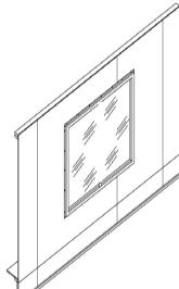
Use caution to avoid covering any window weep holes with sealant, paint or any other obstructive material
