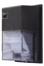
UL wet listed die-cast aluminum construction with borosilicate glass lens or UV stabilized polycarbonate diffuser complete with stainless steel hardware. Mounts to standard 4 inch square electrical junction boxes. Alternate junction box mounting possible via universal mounting ring. Ingress resistant gasket included.
