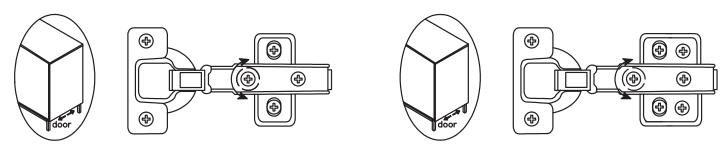
Loosen the side-to-side screws, then screw counter-clockwise to make the gap wider or clockwise to close any gaps.
