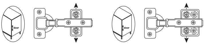
Loosen the height screws, then move the door up or down to make it level.
