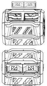
Step6:As shown in the figure on the right, assemble the support "bb"、"cc" and "dd". There are spring buckles at the connecting holes, and the assembly can be completed by inserting the spring buckles into the pin holes.
