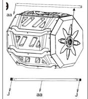
Step8:The whole chamber is installed above the bracket and locked with 2 sets of screws and nuts G, at this time the entire compost machine installation is completed.
