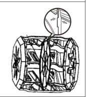
Step5:According to the method of step3, the remaining 4 panels B are continuously installed, and the entire cavity installation is completed at this time.
