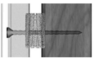
**C** When the shims are properly installed, the frame should not move or twist at all when the screws are tightened and counter-sunk thereby maintaining the 1/8"gap. If there is any movement, loosen the screws and shim tighter to maintain the 1/8"gap, and then re-tighten the screws.
