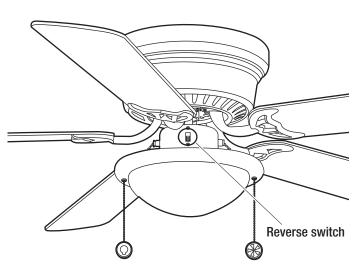
Warm weather - (Counterclockwise Direction) A downward air flow creates a cooling effect. This allows you to set your air conditioner on a warmer setting without affecting your comfort.
