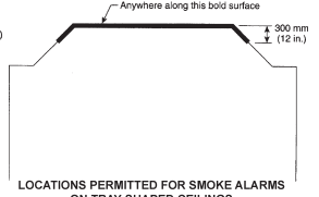
LOCATIONS PERMITTED FOR SMOKE ALARMS ON TRAY-SHAPED CEILINGS
