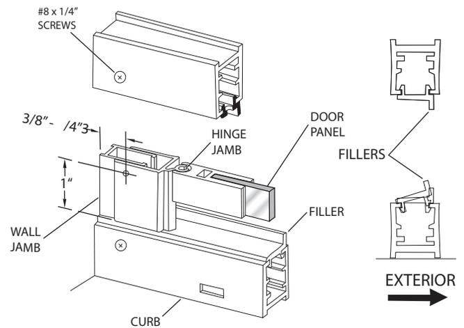
**9** Pull the bottom end of the hinge jamb [L] tight to the curb filler [N] and plumb the jamb. Drill two 1/8" holes thru the hinge jamb and into the wall jamb [B] 3/8" to 3/4" from the wall and approximately 1/4" from the ends of the jamb. Drill a third hole centered between the first two, then enlarge the three outer holes with a 3/16" drill for clearance on the self-tapping screws. Attach the pivot jamb permanently with three #8 x 1/4" truss head screws [K].
