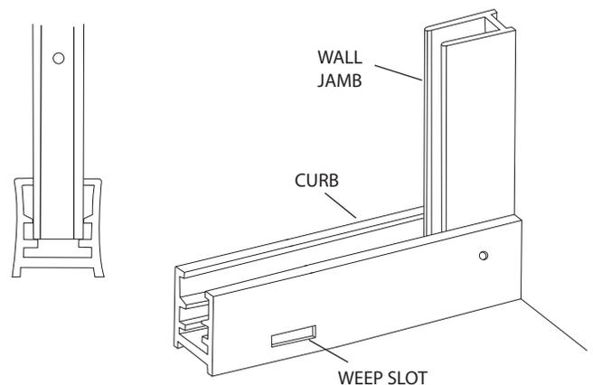
**4** Wipe the shower walls and sill, the curb [A] and the wall jambs [B] with a clean, dry cloth to remove any dust or debris. Apply a 1/4" bead of caulk along the inside of both of the pencil lines marked in Step #2. Carefully replace the curb in the exact position marked. **Caulk the inside of the curb ends where they meet the wall.** Replace both wall jambs and attach to the walls with six #8 x 1 1/2" truss head screws [D].
