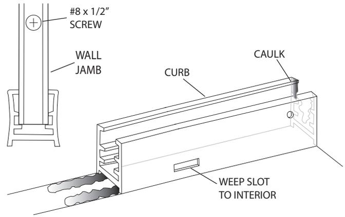
**5** Place two setting blocks [E] into the curb [A] to support the fixed glass panel [F]. Position the blocks 3" from each corner of the glass panel. Set the glass panel into place on the setting blocks and approximately 1/2" into the wall jamb [B]. A strip of masking tape 1/2" from each vertical edge of the glass will aid alignment.
