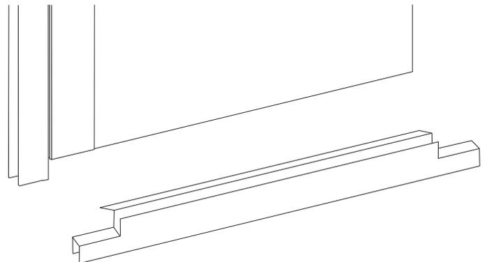
**13** Align the deflector [Q] to the bottom of the door with the hinge side notch over lapping the hinge, then mark the strike side even with the door edge cut deflector at that point.
