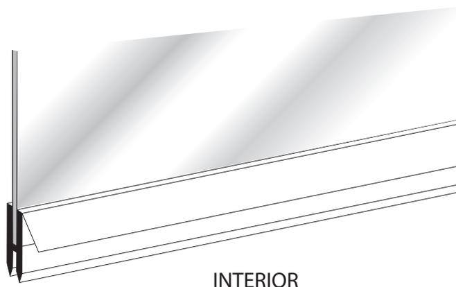
**14** Place the deflector onto the bottom of the door and from inside the shower, close the door and mark the deflector at the edge of the strike jamb. Open the door and remove the deflector. Notch the inside portion of the deflector so the door will close to the strike jamb. Replace the deflector back on the door; close the door to check for clearance.
