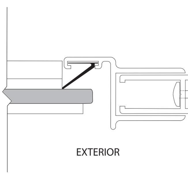
**15** Inspect the pieces of black glazing vinyl, and note the two different profiles. The smaller shape [HH] is installed vertically and the larger shape [JJ] is installed horizontally. For structural strength and maximum water resistance, these vinyls are designed to fit tightly between the glass and framing. To speed installation, use glass cleaner for lubrication and a small block of wood to press the vinyl into place.
