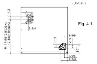
Fig. 4.1. Connection Positions of the Piping
