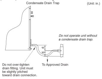
Do not connect the drain pipes directly to sewage pipes, to avoid ammonia odors. The ammonia in the sewage can enter the indoor unit through the drain pipes and corrode the heat exchanger.
