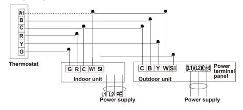
If the matching outdoor (condensing) unit does not have an S1 terminal, then ignore the S1 to S1 connection.
