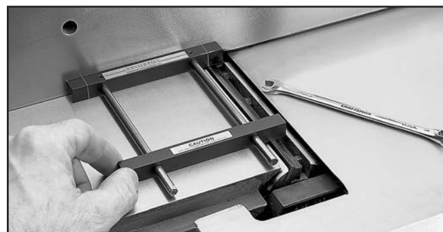
Figure 38. Setting knife height with a Jointer Pal®.
