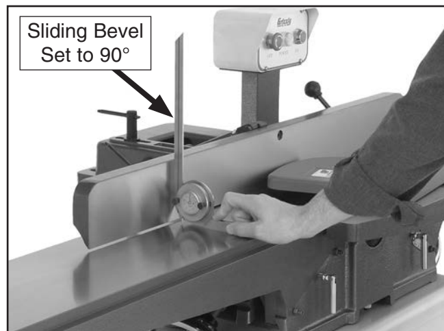
Figure 65. Example of adjusting fence to 90°.
