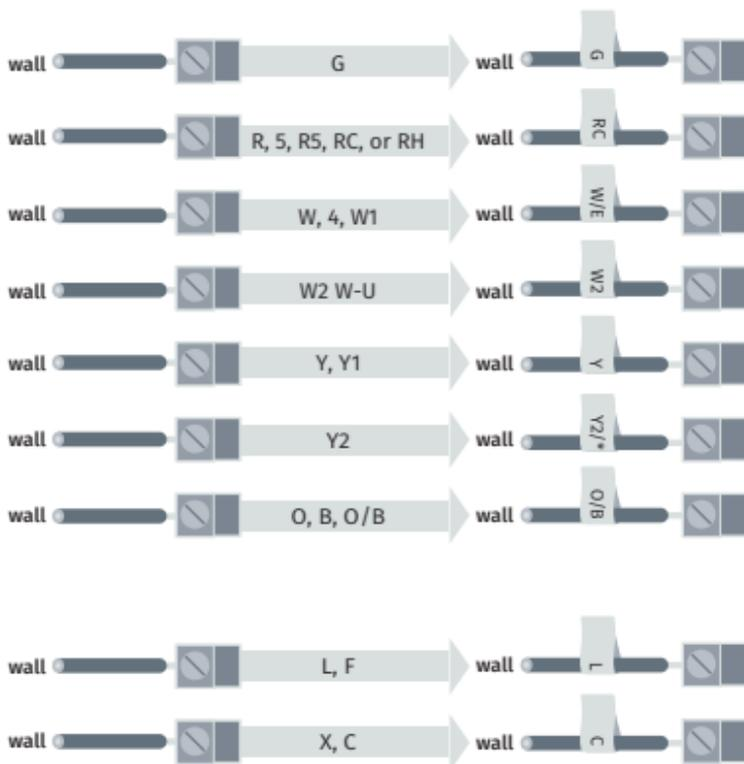
\*Two transformer systems (separate RC and RH wires), clip internal jumper located on back of Sensi above battery compartment.
