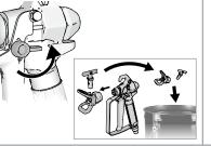
3 Thread Power Flush<sup>™</sup> attachment onto garden hose, turn water on. Rinse paint off of suction and drain tubes, inlet screen and spray tip/guard.
