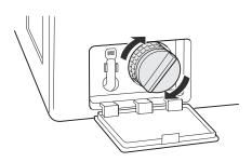
Close the drain pump filter cover.
