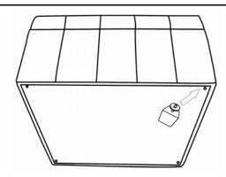
Install the first leg into the bottom of the Storage Ottoman by placing 1 (ONE) piece of plastic washer ring (improves tightness and security of leg) on the threaded stem.
