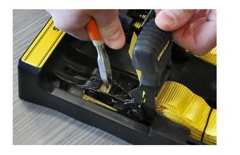
Lift ratchet handle. Find and clip the tie holding the strap in place.
