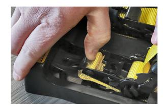
While pulling handle back, lift tab on top of ratchet to release from package.
