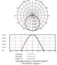
Beam Angle(50%Imax):C0/180Left:54.8 Right:57.4 :C90/270Left:58.7 Right:54.9
