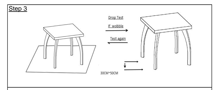
Stand the Table right way up. Place the Table on a LEVEL SURFACE to check for wobbles. If it wobbles, lift the table some 20cm to 30cm high from the ground.
