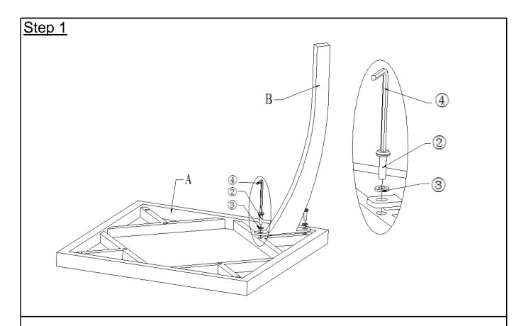
Open the carton and place all the parts onto a clean, non-marring surface. Attach Leg(B) onto the Table Top(A) using Bolt(2) and Washer(3) with Allen Key(4). Only loosely tighten Bolts.
