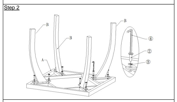
Repeat Step 1 with the remaining three Legs(B). Only loosely tighten Bolts.
