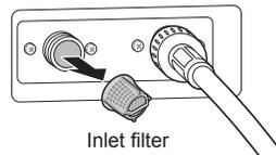
Clean the inlet valve filter or reinstall the water inlet hoses.
