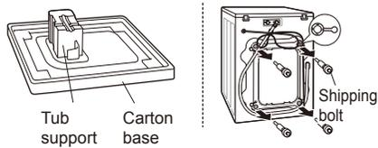
Remove the shipping bolts & tub support.
