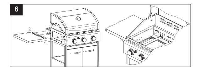
First Assemble the Bottle opener (7) to the left front panel (3) using M4x10mm bolts(JJ). Assemble the M6x12mm to the left front panel, reserve a distance of 5mm. Then fix the left front panel (3) to the body using M5x10 bolts (BB).
