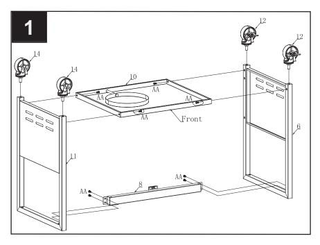
Assemble the back panel (9) to the left cart assembly(6) and right cart assembly (11) using M6x12mm bolts (AA).
