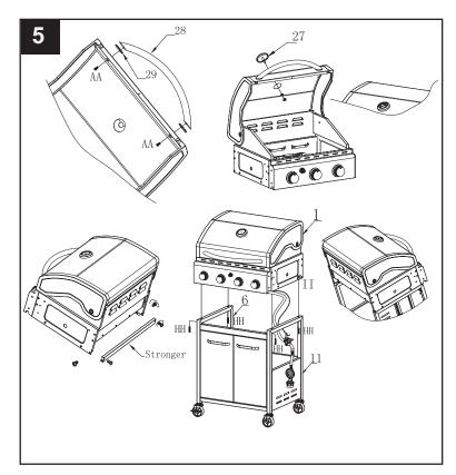
First Assemble the M6x12mm to the body, reserve distance of 5mm. Then fix the left side table to the body using M6x12mm bolts (AA).
