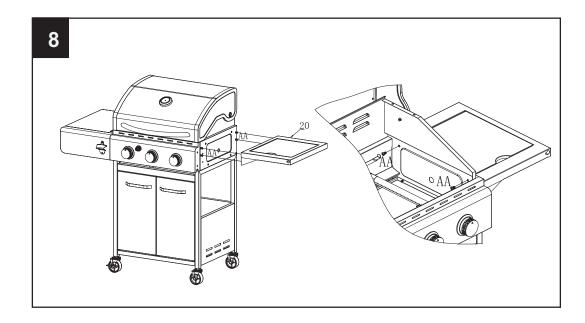
First, assemble the M6x12mm bolt (AA) to the right front panel (21), keep a distance of 5mm. Then assemble the right front panel (21) to the control panel and side burner table using M5x10mm bolts (BB).
