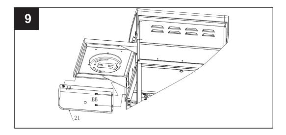
Assemble the side valve and knob base (22) to the right front panel using M4x8mm bolts (GG). First, align to the side valve and side burner (24) then assemble it to the side burner table using M4x8mm bolt (GG).
