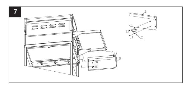
First, assemble the M6x12mm bolts (AA) to the body, reserve a distance of 5mm. Then fix the side burner table (20) to the body using M6x12mm bolts (AA).
