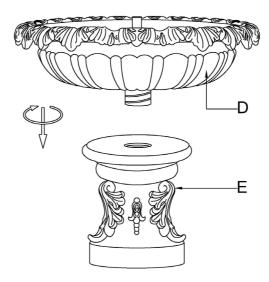
Feed pump cord and light cord through plastic tube, make sure the cords exit out from notch on bottom of base (E).
