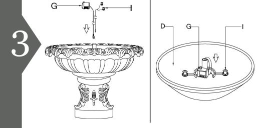
Place lower column (B) into reservoir (D) and twist it clockwise to secure.
