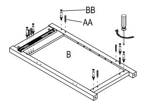
$\hfill\square$  c) Join panel (B) to the assembled body with dowel (AA).
