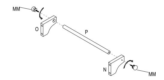
b) Attach towel rack side panels (0) and (N) to the panel (C) with bolt (NN). Turn and tighten bolt (NN) with wrench (00).
