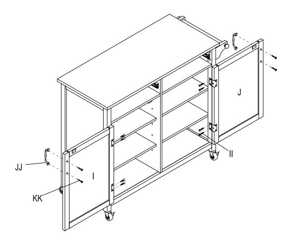
**b)** Attach handle (JJ) to door (I) and door (J) with the bolt (KK).
