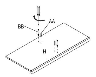
□ c) Join partition (D) to the panel (H) with dowel (AA).
