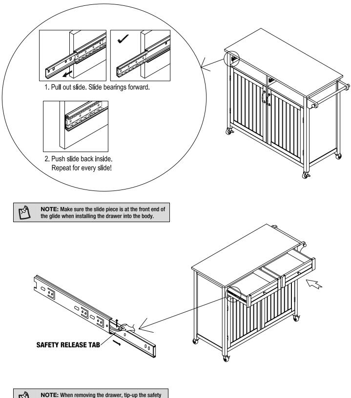
release tab to remove the drawer from the body.
