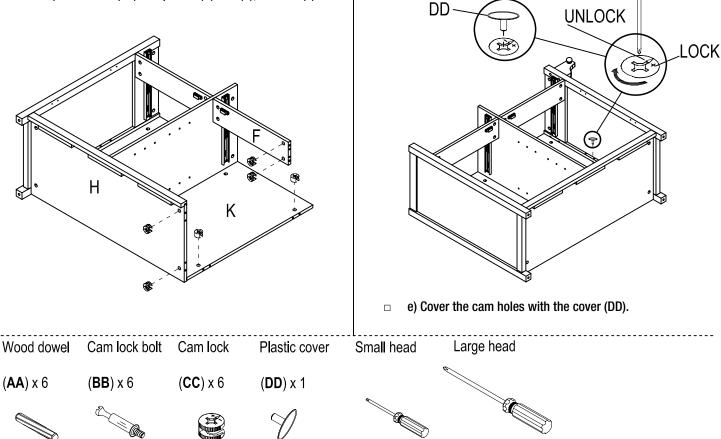
□ b) Insert lock (CC) into panels (H) and (K), and bar (F).
