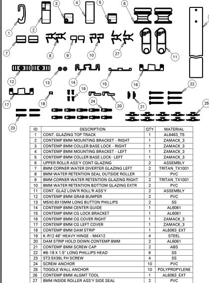
MATERIALS: Anodized Aluminum Extrusions (Track) and Zinc Die Cast (Mounting Brackets).
