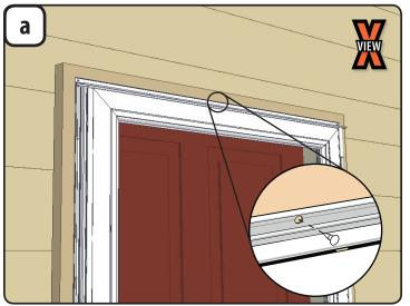
Look at the center hole of the rain cap. If the mounting surface can be seen in the entire hole, proceed to step a2. If the mounting surface cannot be seen in the entire hole, or if there is space above the rain cap, then completely insert the 3/16" plug into the middle hole, then proceed to step b.
