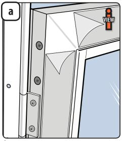
1. Starting at the mitered corners, remove the clear protective tape from both the interior and exterior of door frame, if applicable.
