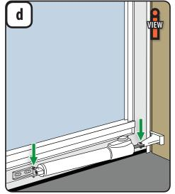
1. Pin bump closer in place using the short pin in the jamb bracket arm and the long pin in the door bracket.
