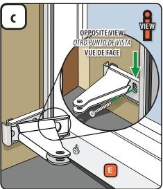
Attach the arm from the installation kit to the base by inserting the tabs on the arm into the slots in the base. Fasten with a 2" screw from the installatio kit.
