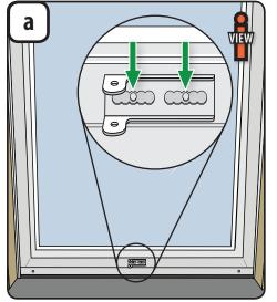
Attach closer door bracket to the door through the two pre-drilled holes using two #12 x 5/8" screws.
