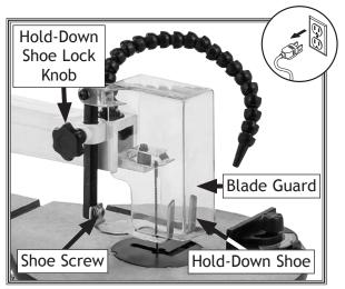
**Figure 18.** Hold-down shoe and blade guard assembly.
