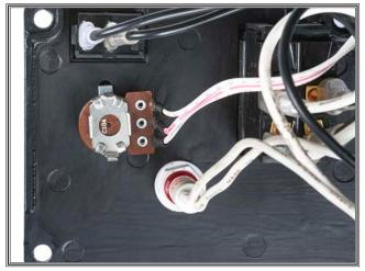
Figure 43. Foot pedal switch & potentiometer.
