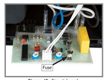
Figure 45. Circuit board.
