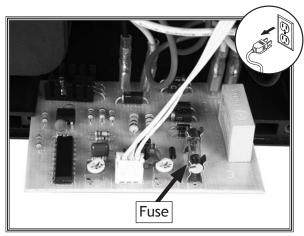
Figure 37. Fuse location on circuit board.
