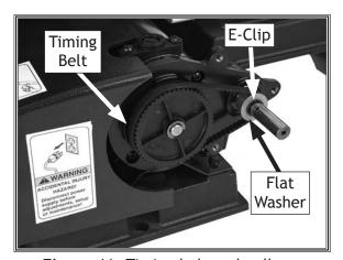
Figure 41. Timing belt and pulleys.
