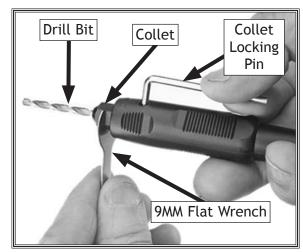
**Figure 14.** Securing drill bit in flex-shaft collet.
