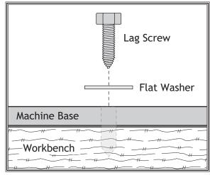
Figure 9. Typical "Direct Mount" setup.
