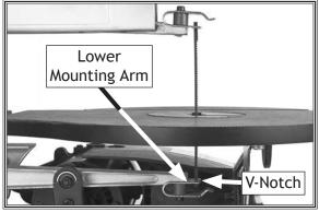
Figure 29. Lower blade mounting arm.
