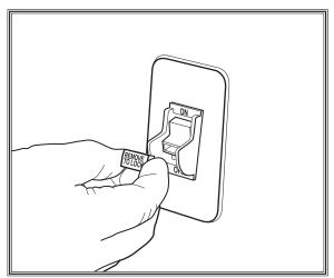
**Figure 17.** Removing switch disabling key from toggle switch.
