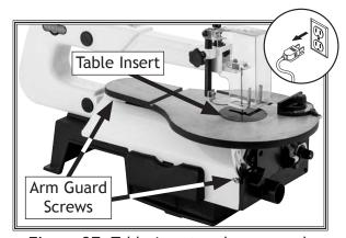
Figure 27. Table insert and arm guard.
