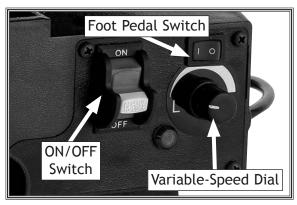
Figure 1. Power and speed controls.
