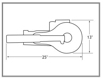
Figure 7. Minimum working clearances.
