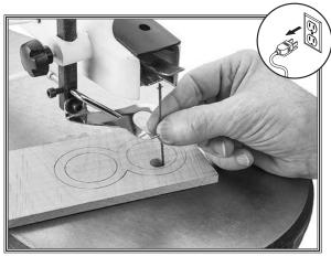
**Figure 23.** Example of installing blade for an inside cut.
