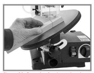
Figure 22. Example of making a bevel cut.
