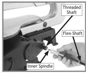
Figure 13. Example flex-shaft installation.
