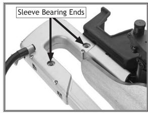
**Figure 34.** Plastic caps removed to expose sleeve bearing ends.
