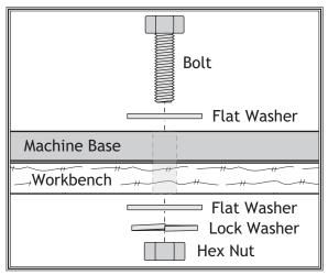
Figure 8. Typical "Through Mount" setup.
