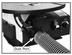
**Figure 15.** Dust port connected to dust collection system.
