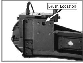
Figure 39. Lower motor brush location.
