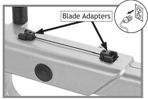
Figure 30. Adapters in indexing slots.
