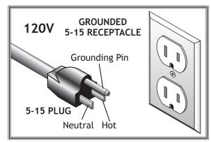
Figure 4. NEMA 5-15 plug & receptacle.
