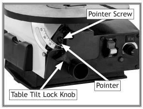
**Figure 35.** Components for calibrating table tilt.
