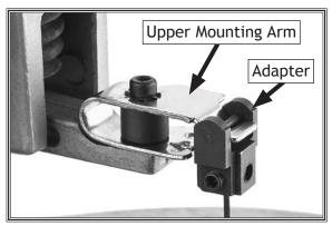
Figure 32. Blade adapter installed.
