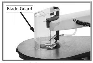
Figure 33. Blade guard position example.
