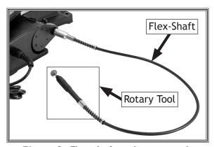
Figure 3. Flex-shaft and rotary tool.
