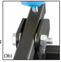
**Step 5.** Install carrier to hitch adapter and stabilizer with M16x90 bolt (J), M16 washers (G), M16 lock washer (H), and M16 lock nut (I). Secure with 1" wrench.
