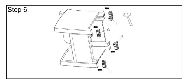
Attach the Left Front Foot Clip(F), Right Front Foot Clip(G), Left Back Foot Clip(H), Right Back Foot Clip(I) to the feet of the Club Chair using the Rubber Hammer(Q) as shown above.
