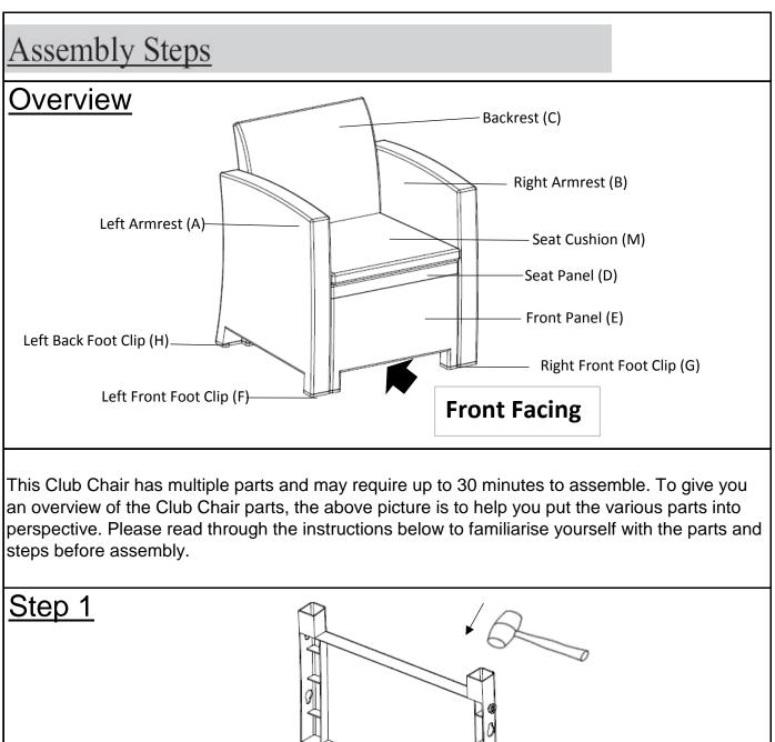
Open the carton and place all parts on a clean, non-marring surface. Place the Seat Panel(D) facedown on the clean, non-marring surface. Insert Front Panel(E) into Seat Panel(D) using the interlocking joints and secure with Rubber Hammer(Q).
