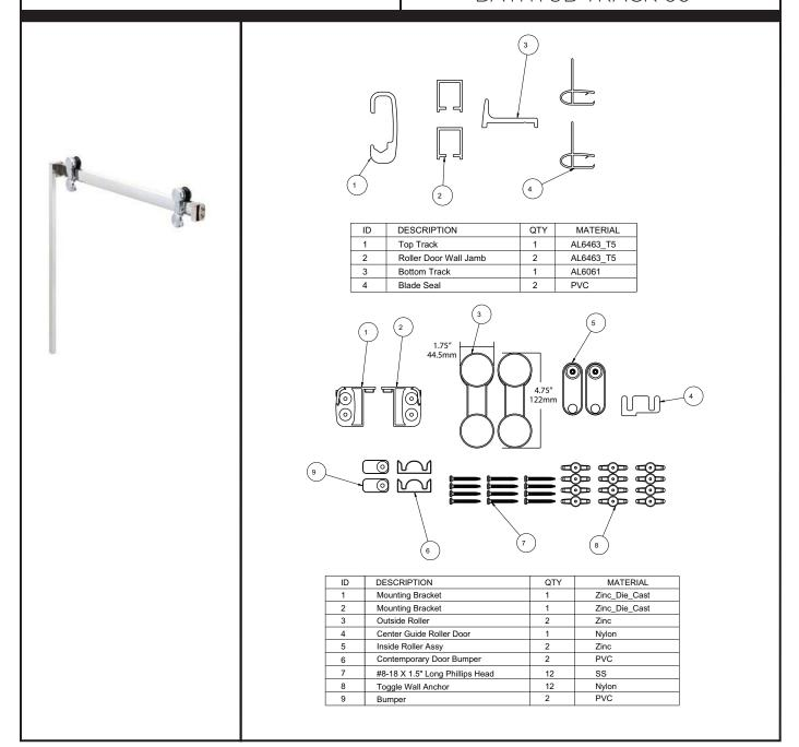
MATERIALS: Anodized Aluminum Excursions (Track) and Zinc Die Cast (Mounting Brackets). Bronze Finish is Powder Coated.
