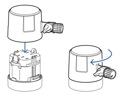
5. Replace the back of the Spotlight and turn clockwise until it locks shut.
