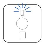
2. The LED light will flash continuously, indicating that it is ready for pairing.
