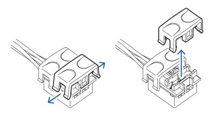
4. Remove the 2 caps from the top of the Controller's Connector. Pull up on the tabs to release the caps.
