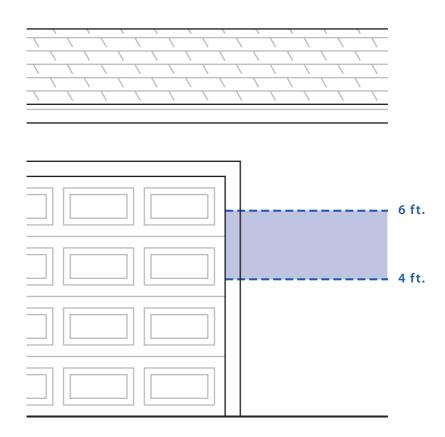
1. Choose a suitable location 4 to 6 ft. above the ground, where you'd like the sensor to detect motion and activate the light.
