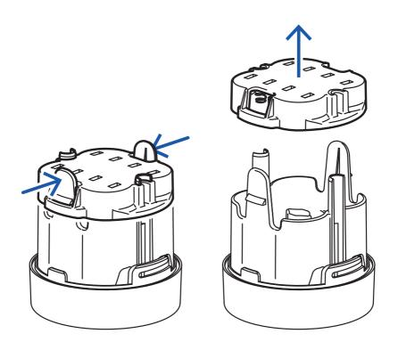
2. Press and squeeze the top and bottom tabs of the compartment cover to open it.
