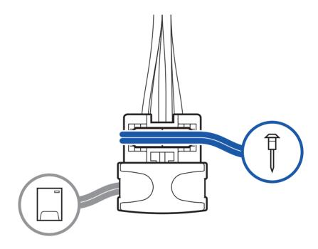
7. Locate the end of the wire leading to the first landscape light fixture in the series. Place it into the channel in the top half of the Connector, marked "To Lights".
