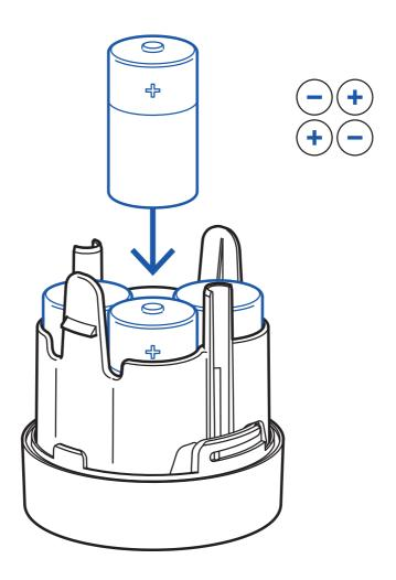
3. Place (4) D batteries into the compartment. Match the polarity markings (+) (-).
