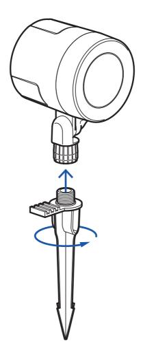
1. Screw the stake onto the bottom of the Spotlight.
