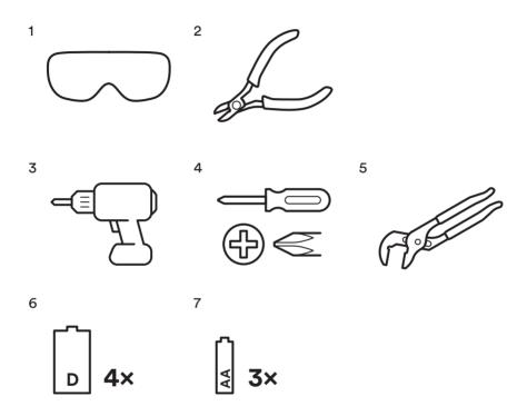
1 protective eyewear 2 wire stripper / cutter (18 to 12 gauge wire)3 drill 4 philips screwdriver 5 pump pliers (optional)
