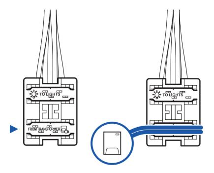
5. Locate the end of the wire leading from the Transformer. Place it into the lower portion of the Connector, in the channel marked "From Transformer". Lead the wire completely through the Connector. Leave the wire's cut end bare or apply an endcap. Ensure the wire is straight and aligned with the channel, and rests on the brass teeth.
