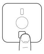
1. Press the button on the front of the sensor unit.
