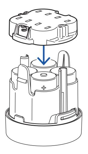
4. Replace the battery compartment cover. Press until it snaps into place.
