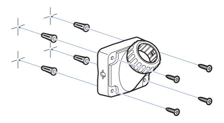
1. Choose a location on the wall 6 to 8 ft. above the ground to mount the Spotlight. Fasten the mount to the wall. Use anchors if needed.
