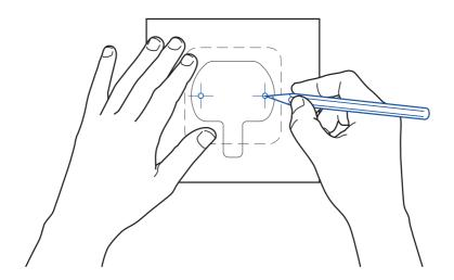
2. Use the enclosed template to mark the location where the sensor will be installed.
