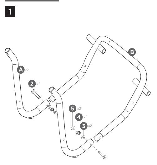
Attach the two part A back frames to the part B front frame with two part 2 bolts, two part 3 washers, two part 4 spring washers, and two part 5 nuts.
