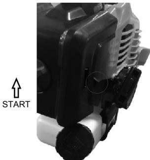
3. Pull the recoil starter handle 3-5 times to start the engine. Hold the machine firmly on the ground with one hand on the power unit, in order not to lose control of the machine during startup as following picture.
