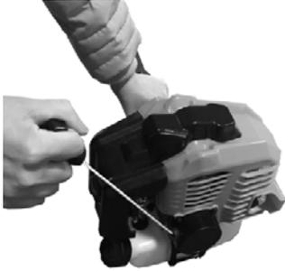
4. Pull the starter grip slowly for 10 - 15 cm until you feel some resistance, then tug it a few times until you hear the engine turn over. Then adjust the choke lever to (RUN) position.
