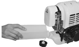
**WARNING! Take care of the emission of exhaust gases. Always shut off engine before fueling. Never add fuel to a machine with a running or hot engine. Take care of fire!**
