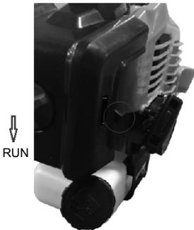
5. Pull the starter grip again until the engine starts as normal.
