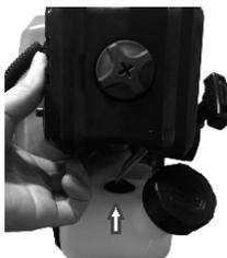
2. Put the choke lever on the (START) position.
